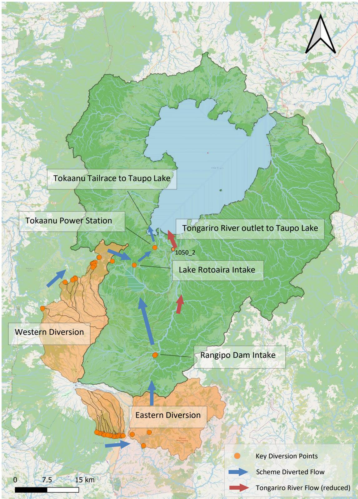
**Figure 3. Tongariro Power Scheme catchments (orange polygon) and structures (orange dots). The natural catchment of Lake Taupō is shown in green. 1050\_2 is the flow recorder at the outlet of the Tongariro River to Lake Taupō.**
