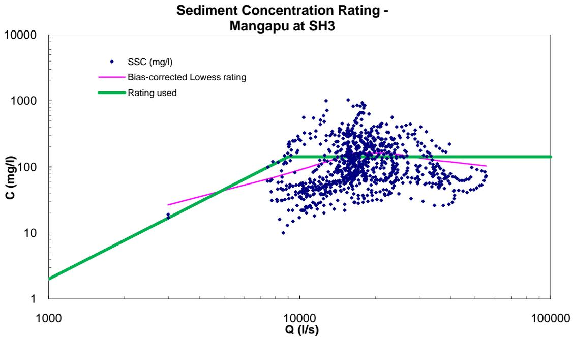
**Figure A-3: Mangapu at SH3 sediment concentration rating.** NB Due to the broad scatter of data at this site, the lowess rating was not considered appropriate. Instead, a simple rating was developed, using the mean SSC for  $Q > 9000$  l/s and, for  $Q < 9000$  l/s SSC tends to 0 mg/l as flow tends to 0 l/s.
