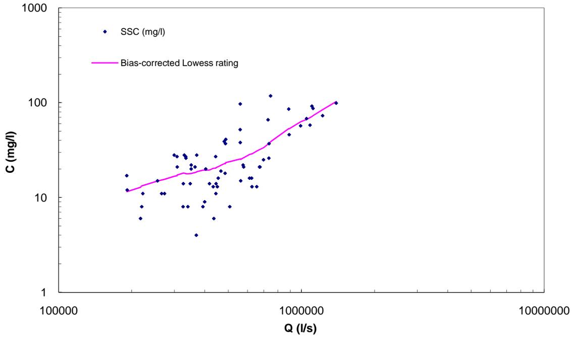
Figure A-13: Waikato at Rangiriri Bridge sediment concentration rating.
