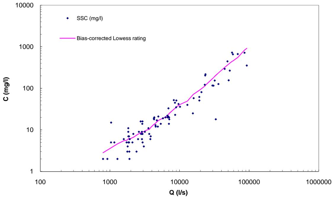
Figure A-17: Mangaokewa at Te Kuiti Pumping Station sediment concentration rating.
