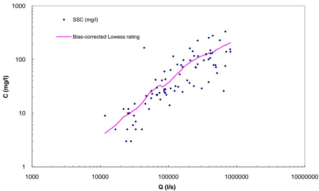
Figure A-23: Waipa at SH23 Bridge Whatawhata sediment concentration rating.
