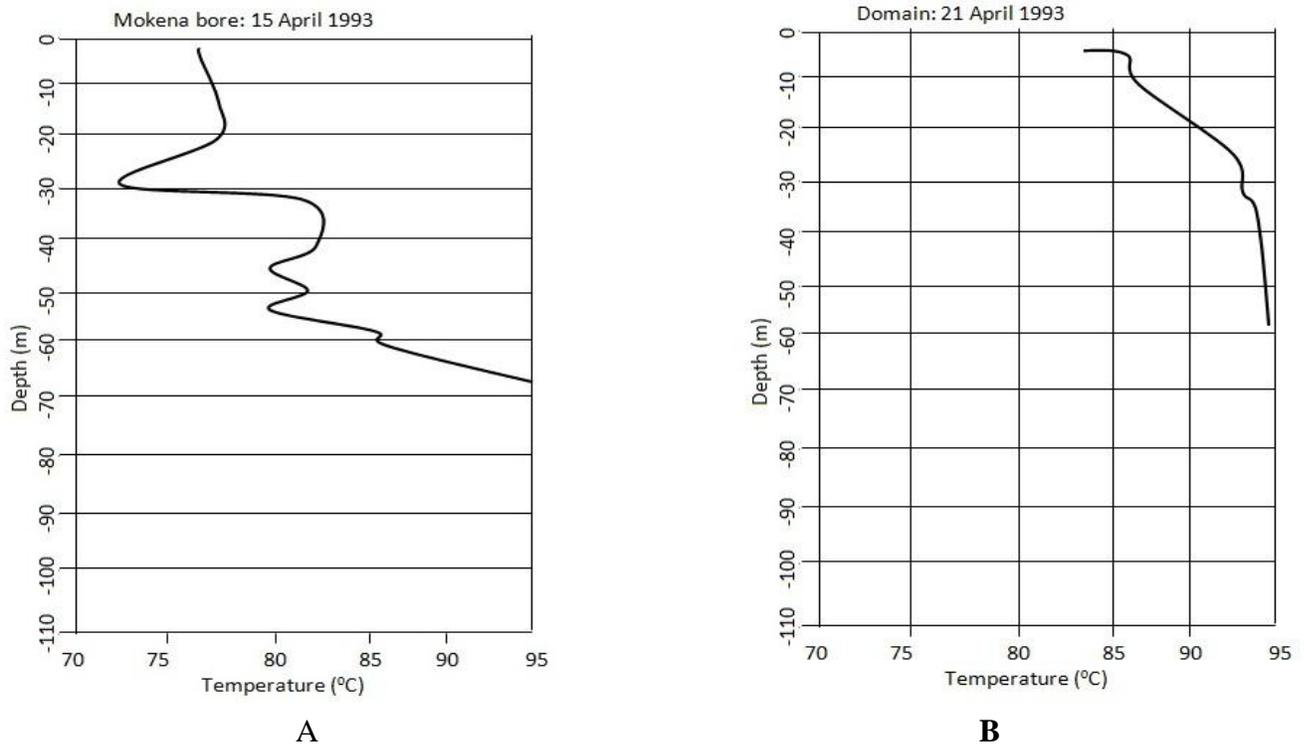
Figure 9. Temperature-depth profiles of Mokena and Domain Trust bores (Michels, 1993).
