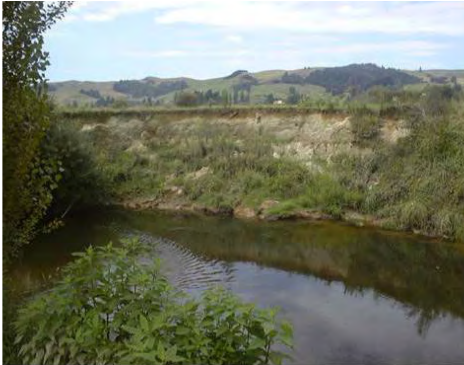
Figure 22: An example of slump erosion; coding and description. Sm (U) o 15 x 2.5 m N: Slump (unstable) outside 15 m long, 2.5 m high, not protected.
