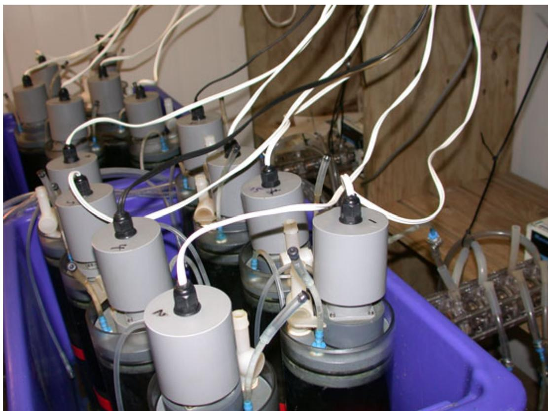
*Figure 5.1.1.* Core incubation set-up with peristaltic pumps visible to the right of the blue basins. The sealed ends of the tubes used to cycle lake water through the cores are clearly visible in the foreground. White taps were used to place the oxygen sensor into the water column and withdraw water samples for nutrient analysis. The cylinders on top of the cores are the magnetic stirrers used to prevent stratification during the experiment.
